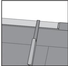
11. Last row. Minimum width 2". Remember to leave a 1/4" expansion gap. Cut the panels lengthwise and glue the short ends.
